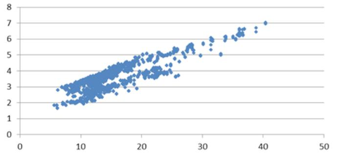
*At 150 MHz different grain types have very similar characteristics, although there are some differences in dielectric constants.*
