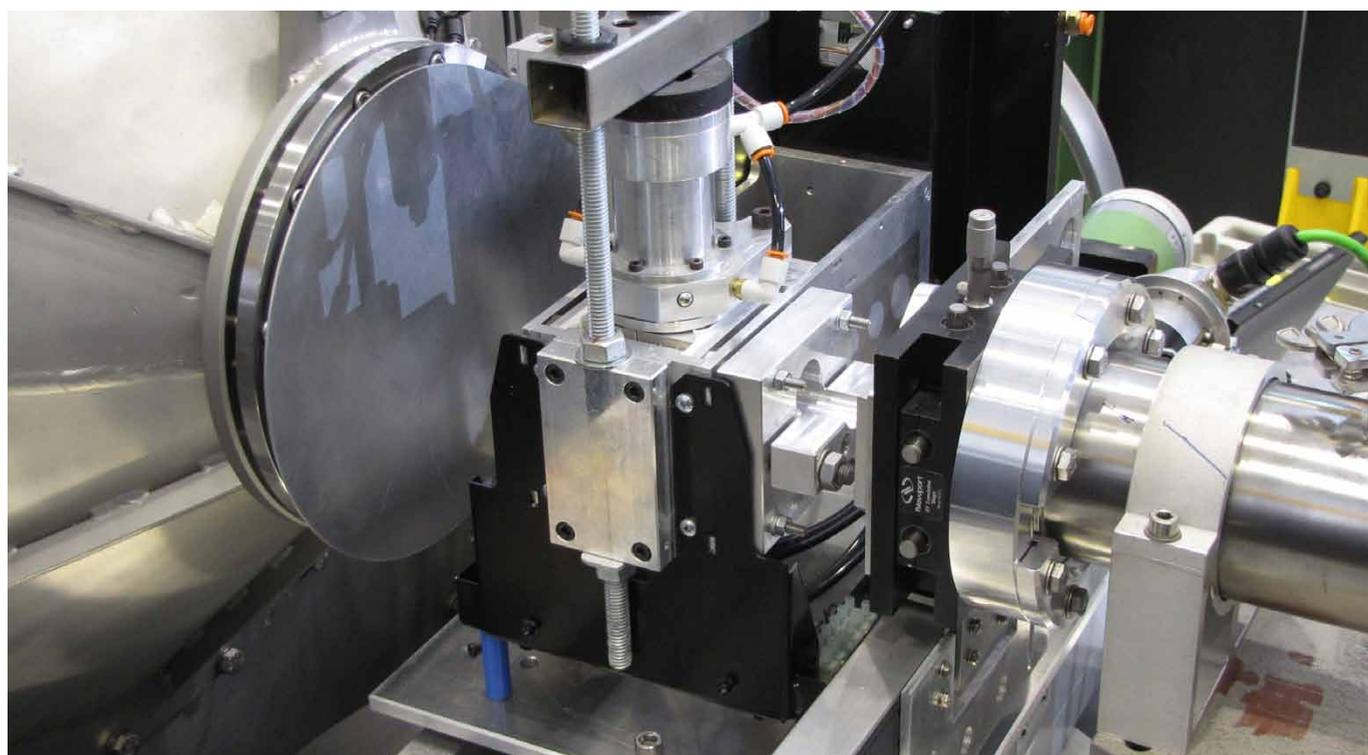
nRVA fitted in the Quokka instrument's beam line.
