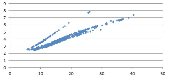
*After correcting for density most of the scatter disappears, and the different grains fall into two groups.*
