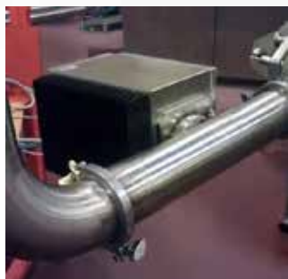
In-line butter measurement
