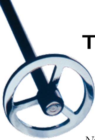
*The Falling Number Method is the worldwide industry standard and accepted method for detecting sprout damage in flour and meal of wheat, durum, rye, barley, other grains and malted cereals. Approved methods include: AACCI/No. 56-81.03, ICC/No. 107/1, ISO/DIS 3093 and ASBC. The Falling Number is the established trading parameter for detection of sprouted grain.*
