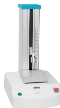
Figure 1: TVT Texture Analyzer
