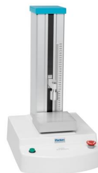
Figure 1: TVT Texture Analyzer
