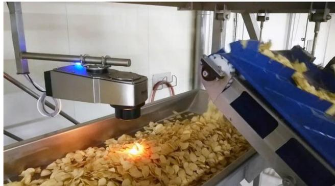
Figure 1 DA 7440 measuring moisture, fat, and seasonings in potato chips
