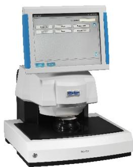
During this time a large number of full spectra are collected and averaged. As the sample is analyzed in an open dish, the problems associated with sample cups are avoided and operator influence on results is minimal. The DA 7250 is IP65 certified and can be placed even in very dusty environments.
