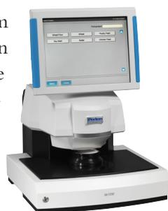
During this time approximately many full spectra are collected and averaged. As the sample is analyzed in an open dish, the problems associated with sample cups are avoided and operator influence on results is minimal.
