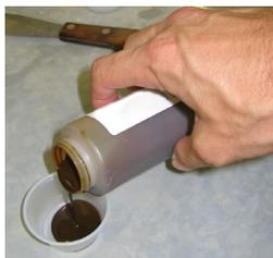
of the DA 7200 is its use of non-contact sampling. Each sample was poured into a disposable sample cup, analyzed, and poured back into the sample bottle. The wet chemistry results were supplied by the manufacturer. Perten Instruments developed calibrations using Partial Least Squares (PLS) regression. Multiplicative Scattering Correction (MSC) and Savitsky-Golay 1<sup>st</sup> Derivative was used as a data pre-treatments to improve the calibration models.
